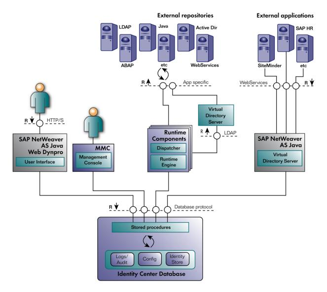
The Identity Center database is used to hold all information about managed users and corresponding account information. All communication between the applications and the database uses the database libraries. In addition, external repositories are accessed from the Identity Center and Virtual Directory Server, to create user accounts and manage access rights. Which systems are accessed, depends on each specific implementation.
